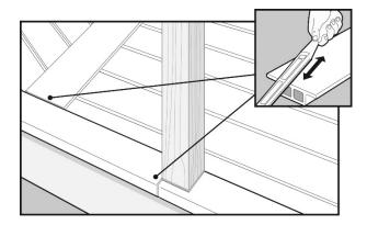
File or route edges when butt joints are unavoidable.
