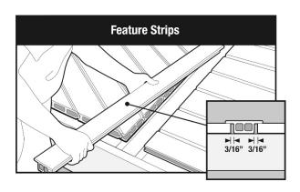
Feature Strips are placed between decking joints.
