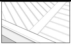
Completed deck after all Feature and Perimeter Strips have been installed.
