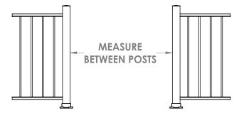
**STEP THREE** - If opening is 40", no cutting is required. If opening is less than 40", deduct 5" from opening measurement and cut panel, leaving equal end spacing.
