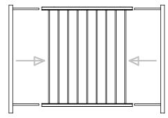
**STEP FIVE** - Drill 16 - 1/8" holes as per diagram and install 3/4" TEK Screws.
