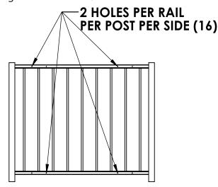
**STEP SIX** - Measure between 1.75" gate posts, deduct 1/16", cut top/bottom snap covers. Once cut, position snap covers over top/bottom horizontal channels and press in place.
