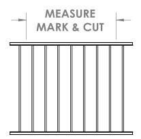
**STEP FOUR** -Insert 1.75" gate end posts into panel upper and lower horizontal channels.
