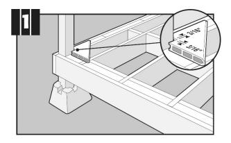
Cut corner piece and attach for guide. Always fasten  $\ensuremath{^{3}\!\!\!/_{\!\!\!4}}\xspace$  from edge of board.
