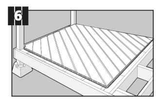
Install Feature and Perimeter Strips when all decking is complete.
