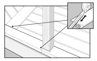
File or route edges when butt joints are unavoidable. To minimize the appearance of expansion and contraction, always butt Perimeter Strips at a post. The joint will be less visible when behind a post and covered with base trim.
