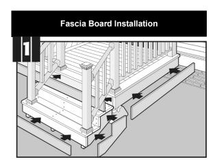
Measure areas to be covered with Fascia. Cut and attach with three fasteners every 12" using same fasteners used for decking. If the Fascia is 6" wide or less, two fasteners every 12" should be used.
