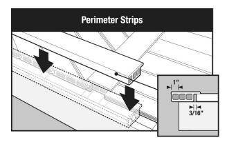
Perimeter Strips are placed around outer edge of decking. Allow for a maximum overhang of 1".
