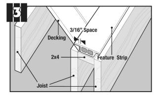
Boards should overlap joist (allowing 3/16" for expansion / contraction) where Perimeter Strips will be added.
