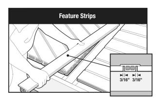
Feature Strips are placed between decking joints.
