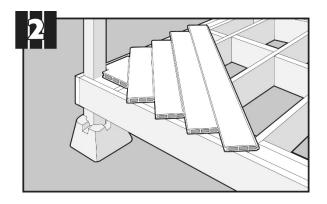
Cut and attach boards as you go. Trim excess *after* all boards are attached.
