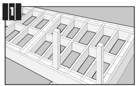
Start decking. Leave 3/16" between house; cover later with siding or molding
