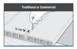
Tongue & Groove boards should be installed with a gap of 1/32" to 1/16". Always use a spacing guide to maintain that spacing. Green Bay Decking has spacing guides available. Call us if your lumber yard does not have spacing tools available. An installation that is not properly gapped will restrict water run-off and may cause buckling, damaging the board and voiding the Green Bay Decking warranty.
