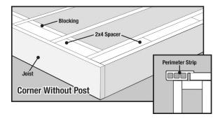
The intermediate joist is the framing necessary for Feature Strips.
