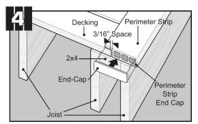
Boards should overlap joist (allowing 3/16" for expansion / contraction) where Perimeter Strips and Feature Strips will be added.
